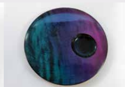
Figured maple disks airbrushed with dye (each with three blended colors) and gloss lacquer.
